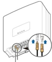
Remove the original PV cable connector and use a new Staubli DC terminal to replace the original one.
